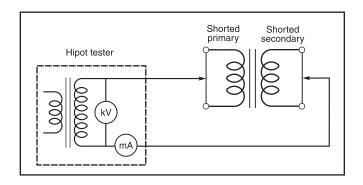
computing. Because magnetic components can be used in multiple applications involving different hazard levels, the hipot test voltage for any specific application must be carefully determined by referring to the pertinent standards for the equipment type.
